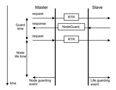
100C-00 Guard time: interval between two RTR messages. Node life time: maximum time available for the encoder to receive a RTR message.
