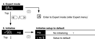
Setup with saved parameters \*"uSEr" is shown only when there is saved parameter by "SAVE" in Expert mode, Refer "Expert mode4-15, Saving user parameter"
