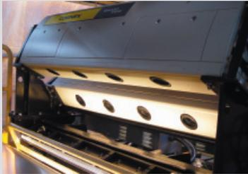
The SmartView Metals system detects irregularities or defects on the surface of the metal strip and then identifies each defect using our patented SmartLearn® multi-step classifier. All information and images are available in real time and can be stored in our database for future use. Reports can be created and formatted to fit the needs of every mill.
