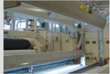
The SmartView Nonwovens system detects, identifies, and displays the irregularities or defects in nonwoven webs made with any process. Finding holes, thin spots, clumps, and other defects allows maximum yield. Finding defects in real time helps avoid adding value to defective material in downstream processes.
