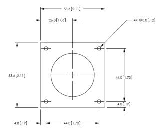
Equivalent for the Diffuser Plate [IC00-DF-SQR56-ISM] and Polarizer Plate[IC00-PL-SQR56-ISM])
