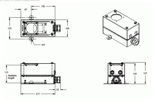
Enclosure is constructed of 16 gauge 316 stainless steel.
