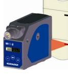
Position the background in front of the sensor light spot and press the SET push-button again. The sensor detects the background and automatically selects the best emission to detect the contrast
