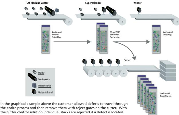
within any layer. This control scenario enables customers to guarantee zero defect product without slowing down the upstream feeder processes.
