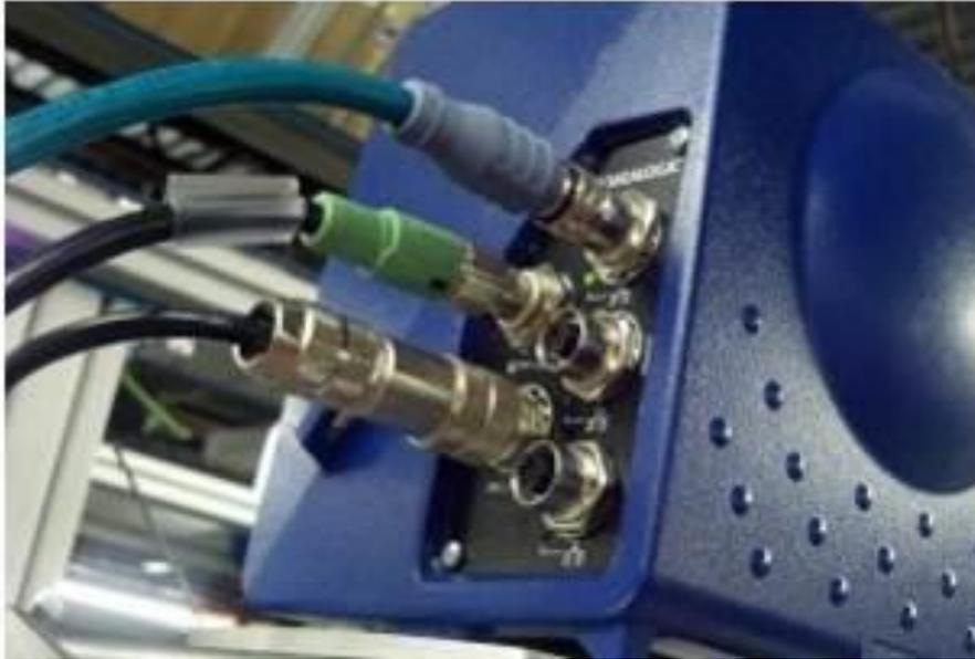
**Figure 16: Connections to the DM3610 Connector Panel**
