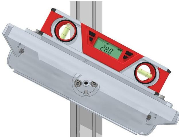
Figure 6: Adjusting the pitch angle
