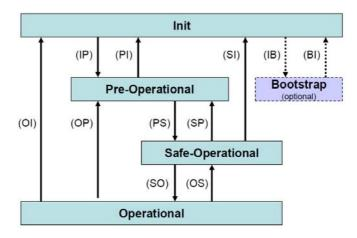
EtherCAT Slave is a state machine; communication and operating characteristics depend on the current state of the device:
