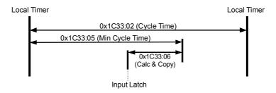
This operating mode has a high sampling jitter (up to 100 microseconds) and can be chosen only when cycle times are quite longer than the jitter if we want to ensure a sufficient real-time system performance.
