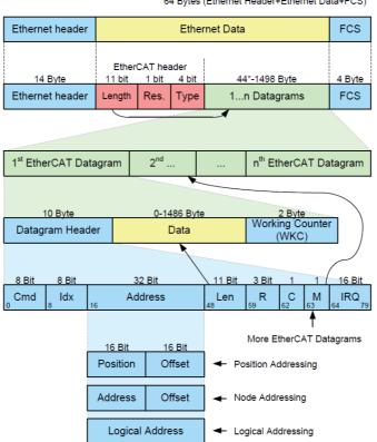
Inside the Ethernet frames data are transmitted among Master and Slaves using PDO (process data objects) protocol. Each PDO message has inside one or more addresses for issuing data to Slaves; data + address/es (and additional elements such as a validation checksum) joined together forms an EtherCAT telegram (Datagram).An EtherCAT frame can contain several telegrams and often a complete control cycle requires more than one frame.
