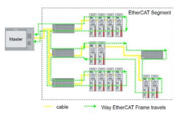
This efficient data flow is guaranteed by the 100BASE-TX full-duplex structure of EtherCAT bus which is fitted with two separated lines for transmitting and receiving data.
