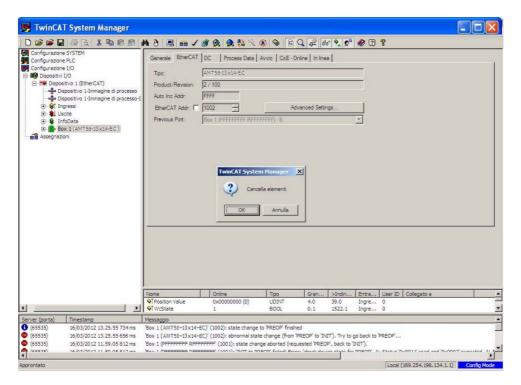
In the left pane of the TwinCAT System Manager main window select and right-click the Device 1 (EtherCAT) item; press the Scan Boxes... command in the menu.
