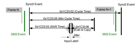
In this operating mode "Jitter" is a fundamental parameter in the sampling of two consecutive data. The main advantage of this mode is that there is a direct relation between the sampling instant and the absolute time of the system; in this way, if we know the shift times of the Slaves, we can have an exact image of the system at a given moment (with a tolerance equal to jitter).
