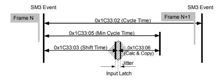
New data will be read by the Master at next cycle (following SM3 event), so if cycle time is too long, data could be relatively old for a real-time system.
