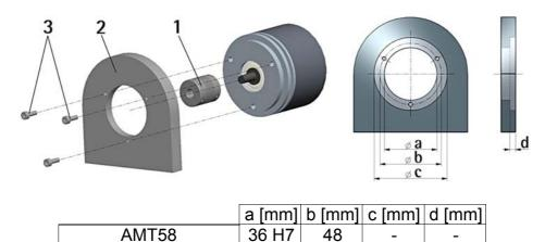
3.1.2 Installation using fixing clamps (code LKM-386)
