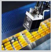
Incorrect occupancy ruled out: The VISOR® Color combines colour and object detection in a single device and can therefore simultaneously inspect occupancy of the blister for completeness and for occupancy with the correct colour.
