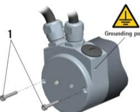
Remove the connection cap to access the terminal connectors and the dip-switches To remove the connection cap loosen the two screws 1. Please be careful with the internal connector. Always replace the connection cap at the end of the operation. Take care in re-connecting the internal connector. Tighten the screws 1 using a tightening torque of approx. 2.5 Nm. Check that the encoder housing and the connection cap are at the same potential before replacing the connection cap!
