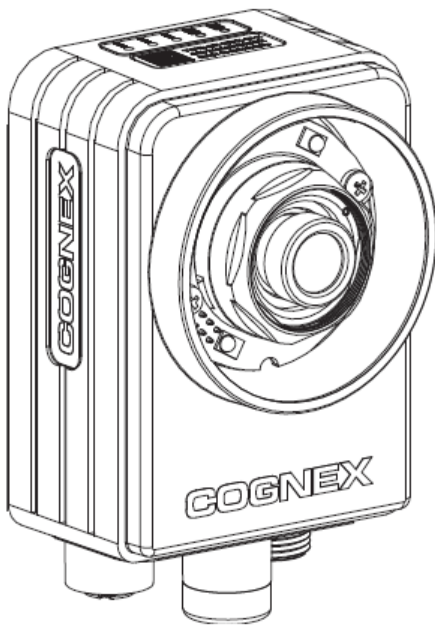
In-Sight 7000 with LED board installed directly on unit
