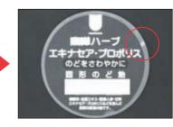
The surface is uniformly lighted to inspect the edge or overlap of transparent film.
