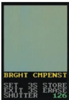
Screen after brightness irregularity correction (There is no irregularity in brightness)
