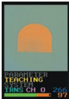
Displays the image screen after correcting position, magnification, and rotation. This is similar to ① **THRU** when there is no correction.
