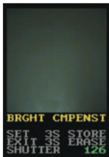
Screen without brightness irregularity correction (There is in brightness)
