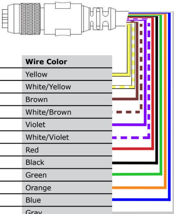
The above drawing shows the **plug** on the device.
