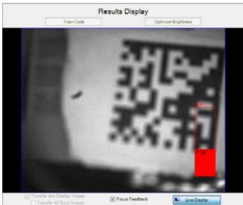
Position the reader in a way that the focus column becomes green. This makes sure that the lens is in focus and you will be able to decode the image.
