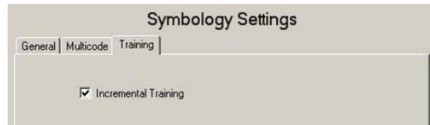
With incremental training enabled, you can train the reader using multiple images showing the symbologies you expect to decode. The reader will train each new symbology while retaining the existing trained symbologies.
