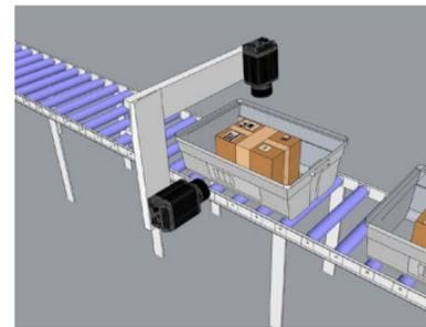
To configure multi-reader triggering, select the **Master/Slave** pane in the Setup Tool (under **System Settings**). For more information, see the *DataMan Fixed Mount Readers Reference*.
