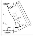
4 Insert the protruded part of fixture to the slit at the lateral side of amplifier (panel mounting mechanism).
