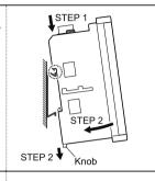
**2** Ensure the amplifier fits perfectly on the DIN rail.
