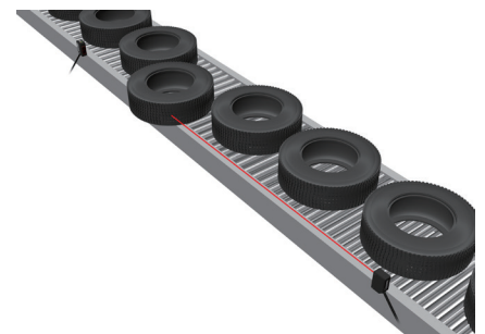
Detecting tires protruding from conveyors (Through-beam type)
