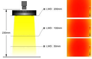
\* This shows the relative brightness distribution when the brightest area is set at 100. The data given here is intended for reference purposes only and is not intended to assure the quality of the product.
