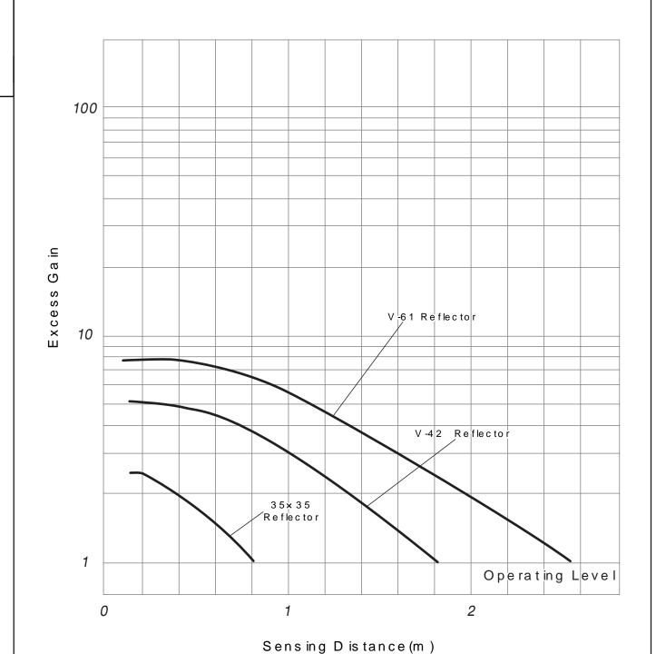
CON.NO QUAN NAME MATERIAL STANDARD DISPOSAL REMARKS DESCRIPTION UNIT DATE **SCALE** SR-150 **A4** 96.10.30 Excess Gain - Sensing Distance APPROVED BY DESIGNED BY CHECKED BY DRAWNED BY ITEM R.Kumo K.Matsumoto S.Nishimura S.Nishimura
