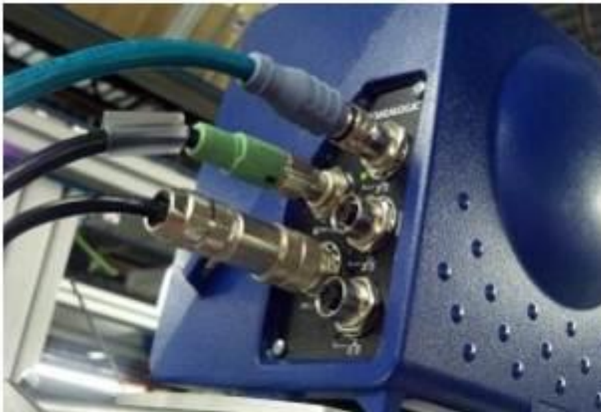
Figure 35: Connections to the DM3610 Connector Panel
