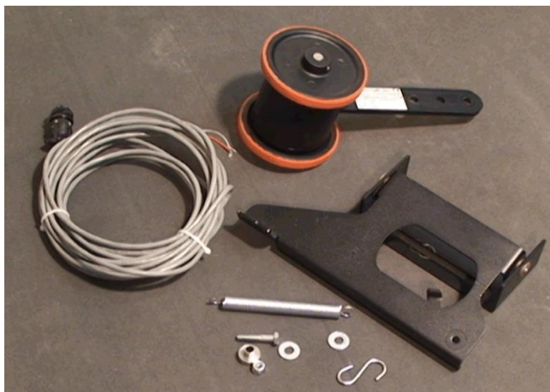
Figure 10: Tachometer, Mounting Bracket, and Cable DM3610 in DWS Systems
