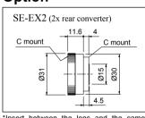
\*Insert between the lens and the camera mount to double the magnification. Note that
