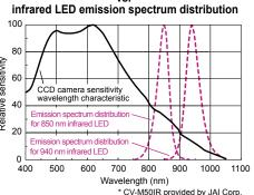
Use a CCD camera sensitive in the near infrared region for use with an infrared light.
