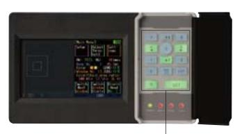
Backlit buttons show which are active to assist in Setup and Adjustment. Help functions can be accessed at any time by pressing the "?" button.
