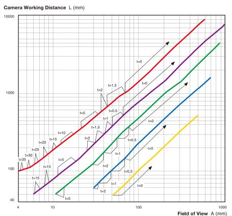
"t=" indicates thickness of Extension ring to use (mm).
