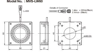
Diffusing plate Model No.: PL-MVS-LW60
