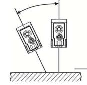
In the presence of moving backgrounds like conveyor belts, especially having a dark or shiny surface, the best object detection performance can be obtained by mounting the sensor at an angle (max 30°) with respect to the horizontal plane, as shown in the figure
