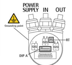
Remove the connection cap to access the terminal connectors and the dip-switches To remove the connection cap loosen the two screws 1. Please be careful with the internal connector. Always replace the connection cap at the end of the operation. Take care in re-connecting the internal connector. Tighten the screws 1 using a tightening torque of approx. 2.5 Nm.
