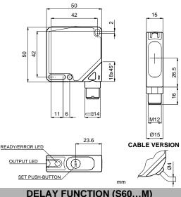
Press the SET pushbutton and keep it pressed until the READY/ERROR LED turns off, blinks and turns off again, then release the SET nushbutton
