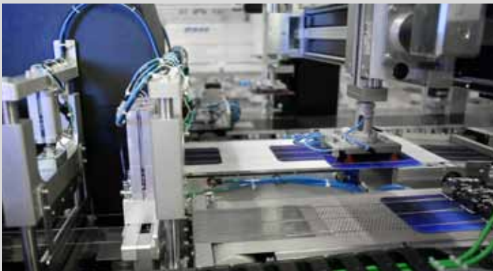
VISOR® Solar sensor for position and edge-break detection.
