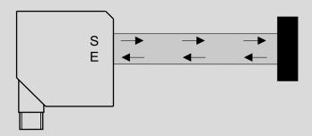
The transmitter and receiver of a proximity sensor are accommodated in a single housing. The light emitted by the transmitter hits the target object, which reflects the light. This returning light is evaluated by the receiver. The advantage of this method is that no reflector is required.
