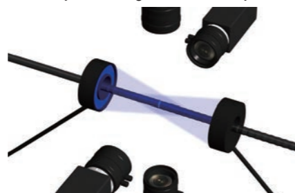
Visual inspection using medical endoscope tubes
