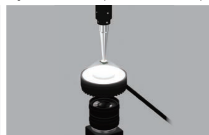
Alignment of electronic components on suction nozzle tips
